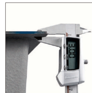
②加厚材料实厚3+0.75以上 Thickened material Actual thickness exceeds 3+0.75mm
